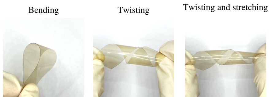
Figure 4-15 Digital photographs of the 40KC/60PV-T45-5R film under deformation forces.
